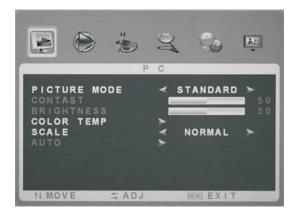
Picture Mode: Select the picture mode. you can choose "STANDARD,DYNAMIC, SOFT,USER" Contrast: Adjust picture contrast. Brightness: Adjust picture brightness. Colour Temp: Adjust picture colour temp: cool, normal, warm mode. Scale Mode: Select picture scale. Auto Adjust: Auto adjust the H Position, V Position, Clock and Phase of the PC signal.
